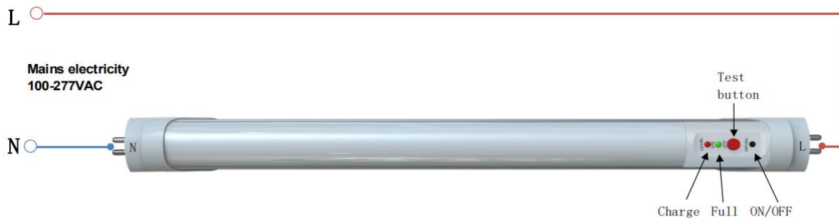
Figure 2. Wiring diagram with a HOT line
